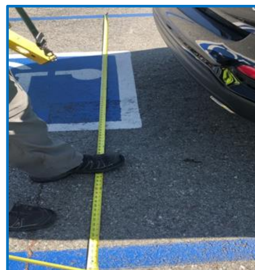
Exhibit B.6: Measured width of parking spaces
